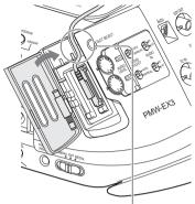
Pass through the cable guide slot.
